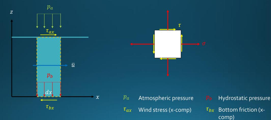
Rate of change of x-momentum of the fluid domain  $\rho h \frac{D\bar{u}}{Dt} = \rho h \left( \frac{\partial \bar{u}}{\partial t} + \bar{u} \frac{\partial \bar{u}}{\partial x} + \bar{v} \frac{\partial \bar{u}}{\partial y} \right) \qquad (15) \qquad \frac{\partial \bar{u}}{\partial z} = 0 \qquad (16)$
